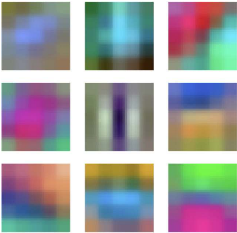
Figure 5-18. A subset of the learned filters in the first convolutional layer of our network
