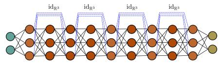
Figure 6.2: Illustration of a neural network with residual blocks.
