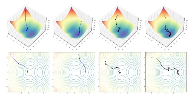
Figure 1.3: Examples of the dynamics of gradient descent (left) and stochastic gradient descent (right) for an objective function with one non-global minimum next to the global minimum. We see that depending on the initial condition and also on fluctuations in the stochastic part of SGD the algorithm can fail or succeed in finding the global minimum.
