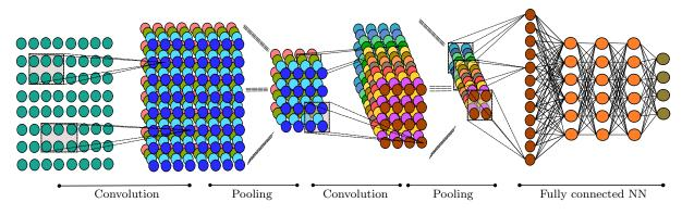
Figure 6.1: Illustration of a convolutional neural network with two-dimensional convolutional blocks and  $2 \times 2$  subsampling as pooling operation.
