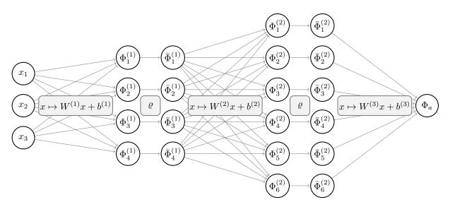
Figure 1.1: Graph (grey) and (pre-)activations of the neurons (white) of a deep fully connected feedforward neural network  $\Phi_a : \mathbb{R}^3 \times \mathbb{R}^{53} \mapsto \mathbb{R}$  with architecture  $a = ((3, 4, 6, 1), \varrho)$  and parameters  $\theta = ((W^{(\ell)}, b^{(\ell)})_{\ell=1}^3$ .
