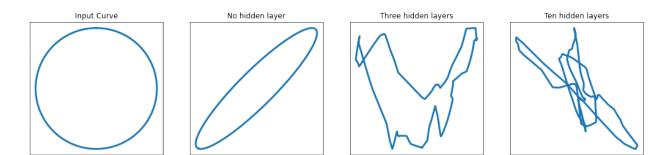
Figure 3.4: Shape of the trajectory  $t \mapsto \Phi_{((2,n,\ldots,n,2),\varrho_R)}(\gamma(t),\theta)$  of the output of a randomly initialized network with 0, 3, 10 hidden layers. The input curve  $\gamma$  is the circle given in the leftmost image. The hidden layers have n = 20 neurons and the variance of the initialization is taken as 4/n.
