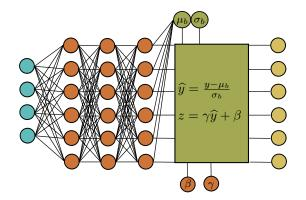
Figure 6.4: A batch normalization block after a fully connected neural network. The parameters  $\mu_b, \sigma_b$  are the mean and the standard deviation of the output of the fully connected network computed over a batch s, i.e., a set of inputs. The parameters  $\beta, \gamma$  are learnable parts of the batch normalization block.
