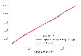
Figure 4.2: Computational complexity as number of neural network parameters times number of SGD steps to solve heat equations of varying dimensions up to a specified precision. According to the fit above, the scaling is polynomial in the dimension [BDG20].
